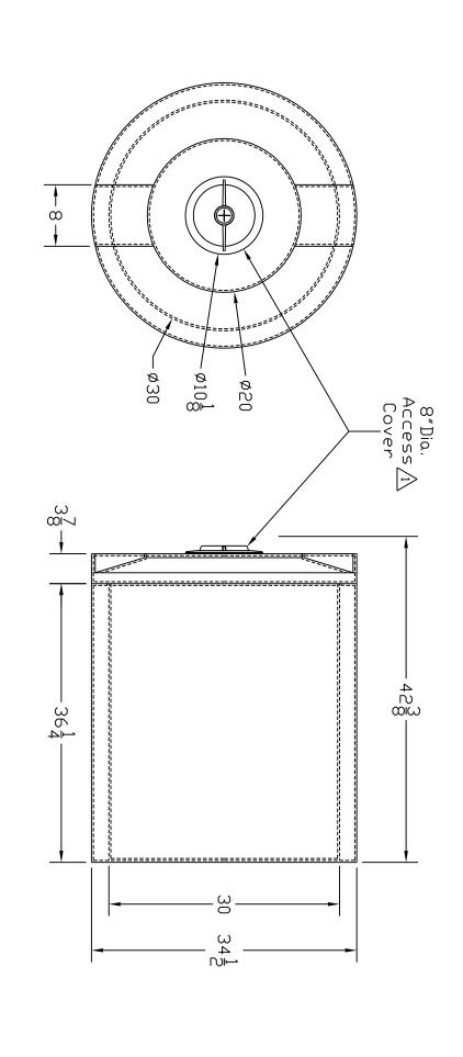
ALL DIMENSIONS SHOWN ARE OUTSIDE PART DIMENSIONS IN INCHES,AND VARY BY THE STANDARD ROTATIONAL MOLDING TOLERANCE OF 2% TO 3%.
